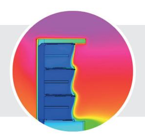
This thermodynamic image (left) shows just how consistently the cold air is held within the Bora cabinet, it is this precise temperature and humidity control that means food is held in the best condition for longer, with less food spoiled.
